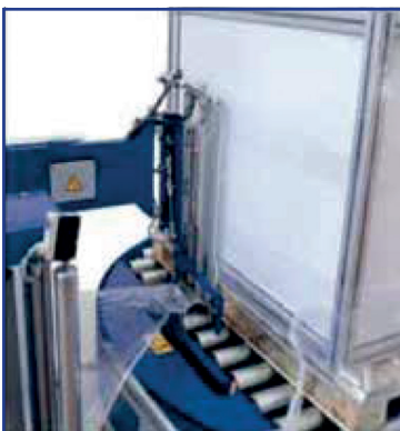
Cutting Unit: Binding film and cutting automatically.
